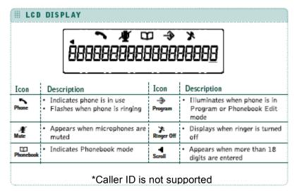
Each Conference Pod is equipped with an LCD display and uses Icons to assist in conference processing.
